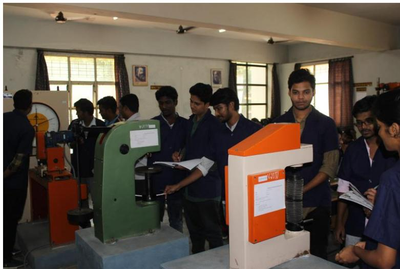
The machines and equipment used to determine experimental data include universal testing machines, torsion equipment, spring testing machine, compression testing machine, impact tester, hardness tester, etc. Data will be collected using Dial indicators, extensometers, strain gages and strain indicator equipment, as well as load and strain readouts on the machinery and graphing capabilities to print relevant plots for analysis.
