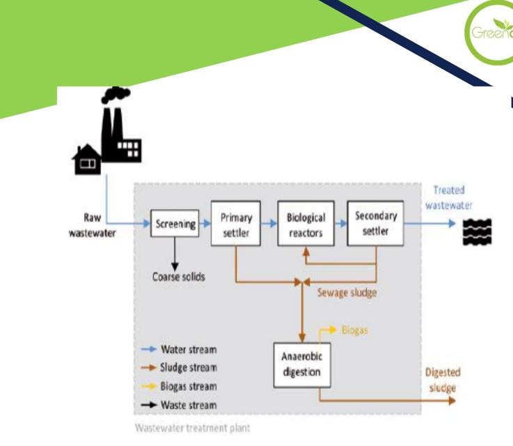
**The physical process**: this is the mechanical treatment of the water that involves removal of debris from the raw wastewater right from the point it enters the plant. The screening and primary settling of debris. Wastewater enters the treatment plant through the inlet chamber from where it is channeled to the coarse screen that removes solid waste.
