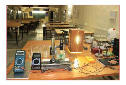
Refractive index sensor setup
