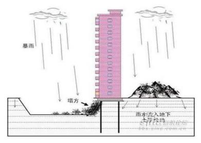
Schematic representation of failure of building in Shanghai in China (Subramanian, 2009)
