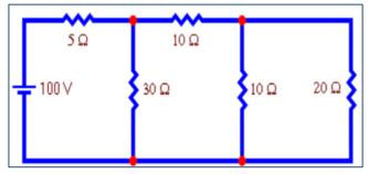
Use nodal analysis to find the voltage at each node of this circuit
