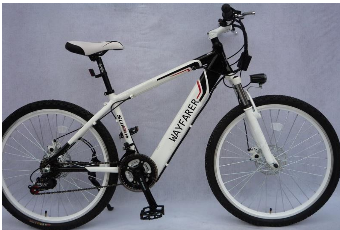
Fig 4.1.1: e-bike where battery is hidden inside frames (just for evidence)
