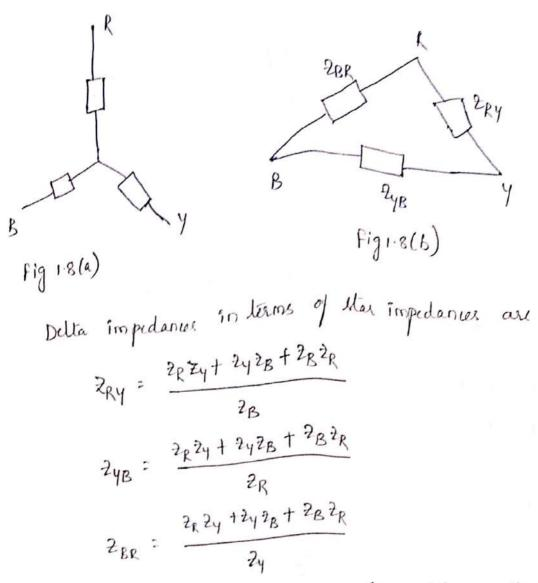
The converted network is shown in fig 1.8(6). Similarly we can replace the della load of Fig 1.8(6) by an equivalent star load with branch impedances as
