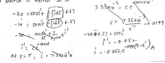
$$\Rightarrow \text{ For the Circuit Mouon in figure, determine the transient current when the kwitch is moved from position i to 2 at t=0. The circuit is in Atady date with Revited in position 1.
