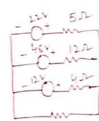
From given network we can write,  $V_1 = 12V$ ,  $V_2 = 48V$ ,  $V_3 = 22V$ 2,=42, 22=122, 23=52 4, = 1 = 0.20, 42 = 12 = 0.0830, 43= 1=0.200  $V_{m} = \frac{V_{1}Y_{1} + V_{2}Y_{2} + V_{3}Y_{3}}{Y_{1} + Y_{2} + Y_{3}} = \frac{12 \times 0.257 + 48 \times 0.083 + 22 \times 0.25}{0.257 + 0.083 + 0.257}$ = 24 21.35V
