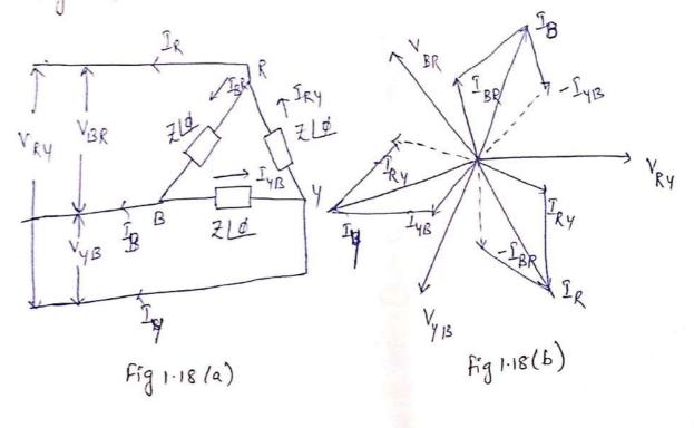
If the load impedance is ZLD, the current flowing in the
