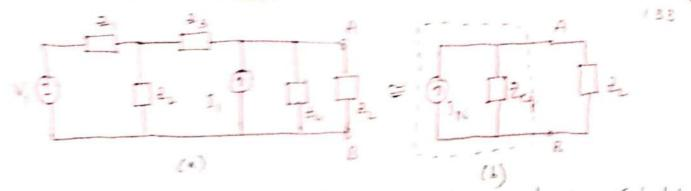
For obtaining cussort In their the bad terminals A-R Calculate the current thereagh the short circuited path by using any of the metanot templetication techniques, This is Nortonic current In It is shown in Fig below
