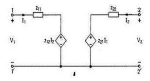
Equivalent circuit of the two-port network in terms of Z parameter.
