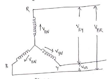
Fig 1.10 Similarly VyB means that Y is positive with respect to point B during its positive half cycle, it also means that  $V_{RY} = -V_{YR}$ .
