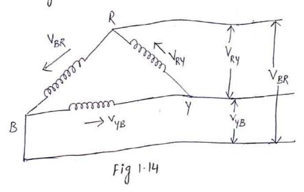
From the manner of interconnection of three phases in the Circuit, it may appear that the three phases are short circuite among themselves. However this is not the Case. Since the system is balanced, the sum of the three Voltages round the closed mesh is zero; consequently no current can flow around the mesh when the desiminals are open.
