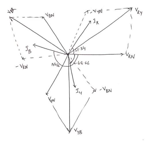
→ A balanced 3-phase system supplied from 400V, 50H 2 supply Mas R, L & C elements connected parallel in each phase. The values of R, L & C are 10-2, 1H & 100/1F supertively Calculate the line Current. The power & power factor
