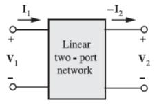
Terminal variables used to define ABCD parameters
