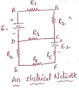
Node: A point at which two or more elemente are joined together is called a node. The junction pointe are also the modes of the network. In the network shown in the Fig. A, B, C, D, E and F are the nodes of the network.
