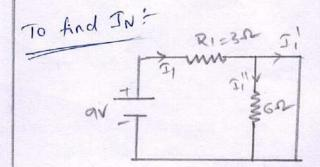
Due to short circuiting the load terminal, arrent does not flow through Gal resistor.
