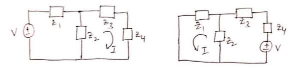
In other words, the vand I are mutually transferable. The ratio  $\stackrel{\vee}{\pm}$  is Called transfer impedance where v is voltage introduced in loops and I is the response due to V in loop 2 Proof of Reciprocity Theorem:-
