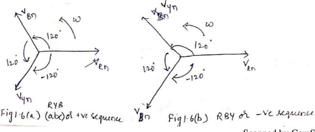
$V_{Rn} = V_p Lo$   $V_{yn} = V_p \frac{L^{120}}{L^{240}}$   $V_{Bn} = V_p \frac{L^{-240}}{L^{240}} = V_p \frac{L^{130}}{L^{130}}$
