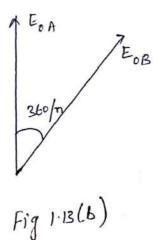
The angle of phase difference between adjacent phase. The Voltages is  $360^{\circ}/m$ . Let Eph be the voltage of each phase. The line Vollage i.e., the Voltage between A and B is equal to  $\lim_{R \to S} = E_{L} = E_{RO} + E_{OIS}$ . The vector addition is shown in fig. 13(c)  $E_{RIS} = E_{L} = E_{RO} + E_{OIS}$ . The vector addition is shown in fig. 13(c) It is evident that line current and phase current are same
