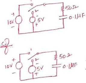
Given that Given that When switch is at position 1, steady When switch is at position 1, steady when switch is at position 1, steady state is reached. Therefore Capacitor state is open circuited and charged to lov  $V_c(\bar{o}) = 10V$ ,  $i(\bar{o}) = 0A$
