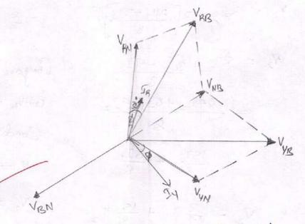
from the phasor diagram, it is clear that the phase angle blu VRB and IR is (20°-0) WI=VRBIRCOS(20°-0)
