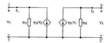
Equivalent circuit of the two-port network in terms of Y-parameters
